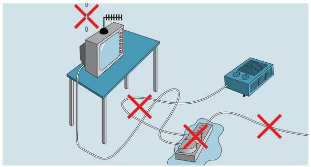
Avoid excessive cabling inside tents and keep all electrical appliances and connections away from water
